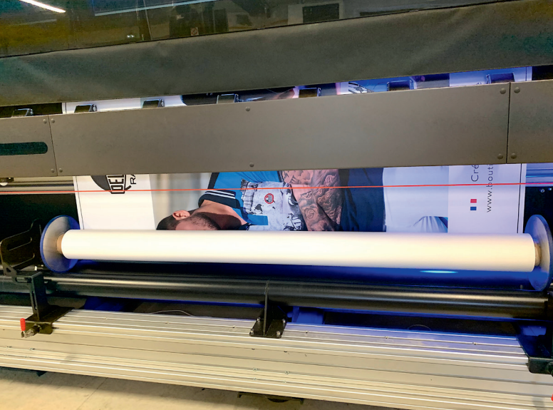
Aveline's VUTEk 3r+ printer is configured with four colours, plus white, and is used to print everything from micro-perforated wraps to 4x3-metre blue back paper, to double-sided posters, and unique projects such as kakemono Japanese hanging scrolls.
