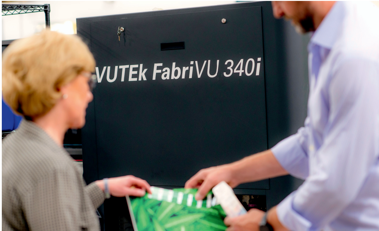
Maverick Concepts has developed a unique process that enables its team to use the VUTEk FabriVU 340i to print on transfer paper and then sublimate offline to rigid substrates.
