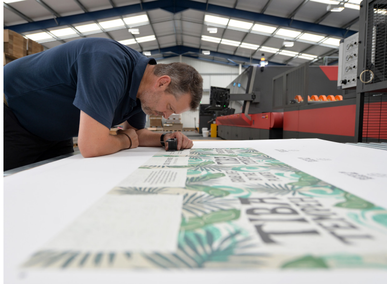
The unique 1.8 x 3 metre capacity of the Nozomi C18000 LED corrugated digital press, its single-pass format, its ability to print 75 linear metres per minute, and its white ink capabilities were all major draws for Durham Box.
