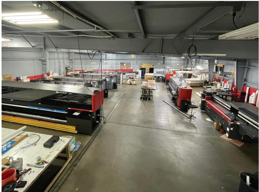
The GCI Digital Imaging team's production floor now includes two EFI VUTEk Q5r roll-to-roll printers, a VUTEk h5 hybrid printer, and two EFI VUTEk GS3250LX Pro hybrid printers.
