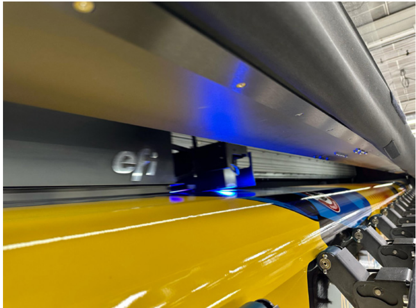
EFI's UltraClear Coat installed on Indy Imaging's VUTEk Q5r printers print inline, simultaneously with the image, and can be used for decorative, high-quality effects on prints or as a final coating to help protect graphics.
